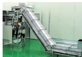
Covered inclined conveyor
