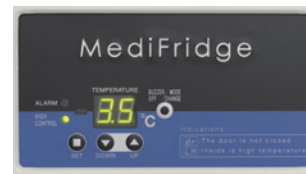
HC (High Control) mode Indicates the temperature from 1°C to 7°C by the unit of 0.1°C.
