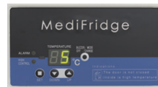
EC (ECO Control) mode Indicated by the unit of 1°C
